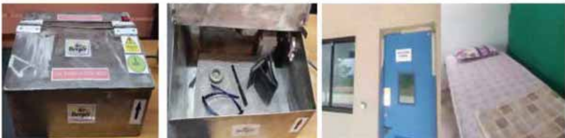
In-house fabricated UV Sanitization box for sanitization of employees' personal belongings
