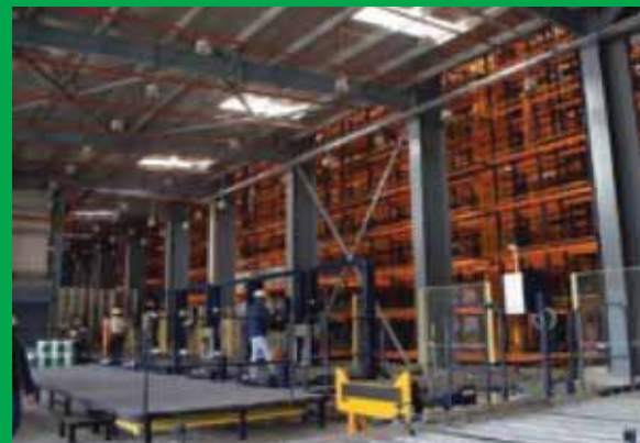
ASRS for faster and man independent storage and retrieval
