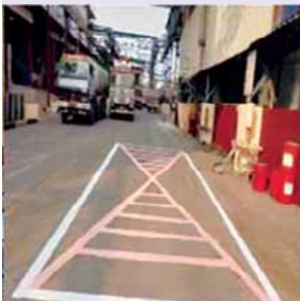
Color coding of parking place near to specific monomer storage tank at unloading point
