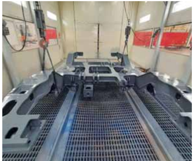
VANDE BHARAT BOGIE of Indian Railways is being painted with Berger Fluoro paint system. Berger Paints is the 1st company approved by RDSO for Fluoro Paint System as per Japanese JIS specification. This is one of the prestigious projects where RDSO and Indian Railways have appreciated our product and services.
