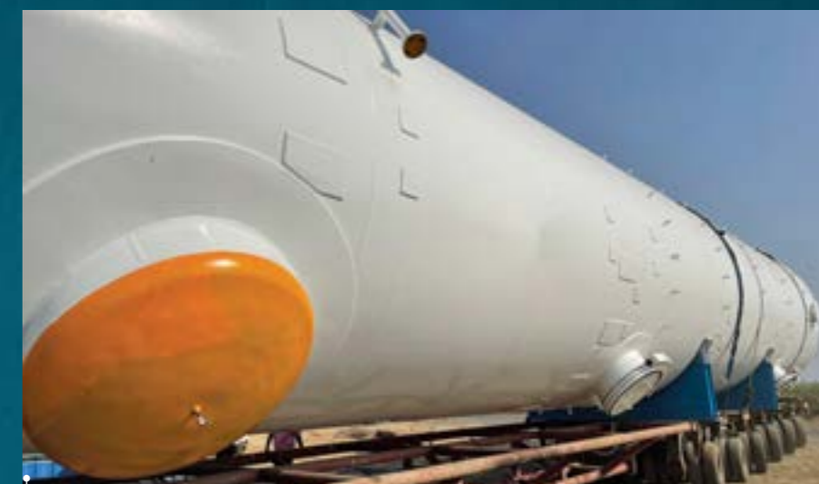
Epilux 45 ZNPH, a Universal Primer used in this project is a special anti-corrosive base coat which is recommended for a variety of substrates and in this coating system, we have a high gloss Bergerthane as a topcoat.
