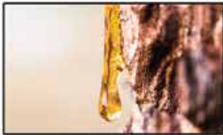
Resins in wood try to leach out
