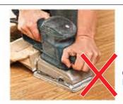
Cross grain sanding leads to veeners grains being damages
